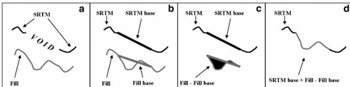
Fig. 3. Illustration of the process used to merge the two elevation surfaces. For the void area in the SRTM model and for the corresponding region in the fill surface (a), TINs are calculated from points at the edges to create base surfaces (b). The fill base surface is then subtracted from the fill surface (c) and added on top of the SRTM base surface (d) to obtain a seamless DEM.
